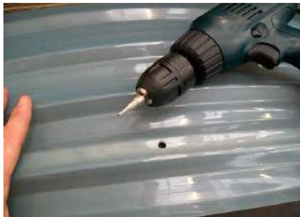
Locate the pilot hole in the top of roll cage, and transparency to perform pre-drill of cover (diam.10)
