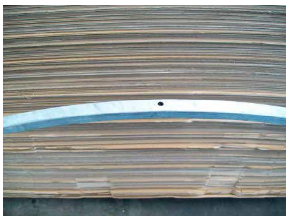
Locate the pilot hole in the top of roll cage, and transparency to perform pre-drill of cover (diam.10)
