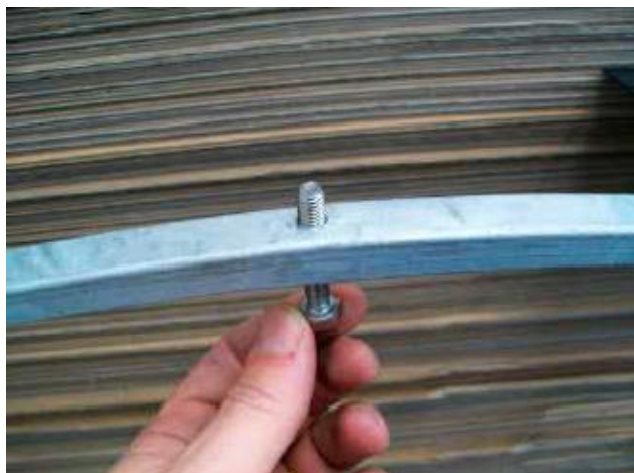
Insert the M9x45 screw
